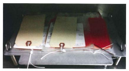
Position the temperature probe so that it rests in between the thickest portions of two freezing bags. The probe must not come in contact with the metal of the freezer press. Place the top plate of the freezer press onto the rack and clamp it in place to hold the bags securely on the press.
