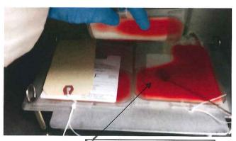
Temperature probe being "sandwiched" between two (2) cryopreservation bags
