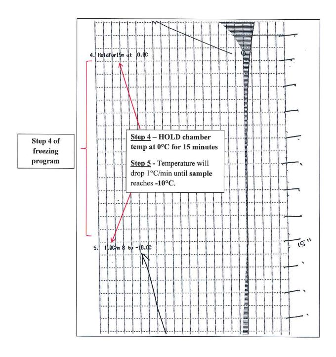
Step 5 – Temperature will drop 1°C/min until sample reaches -10°C.
