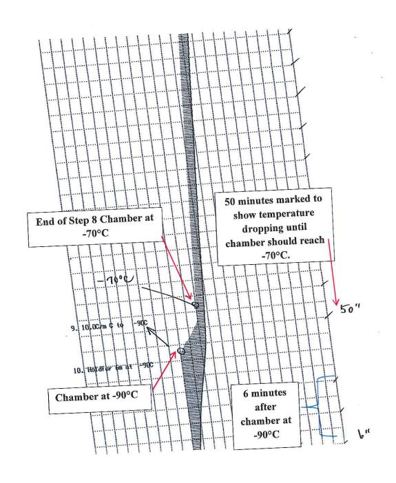
Step 9 – Temperature will drop 10°C/min until chamber reaches -90°C.
