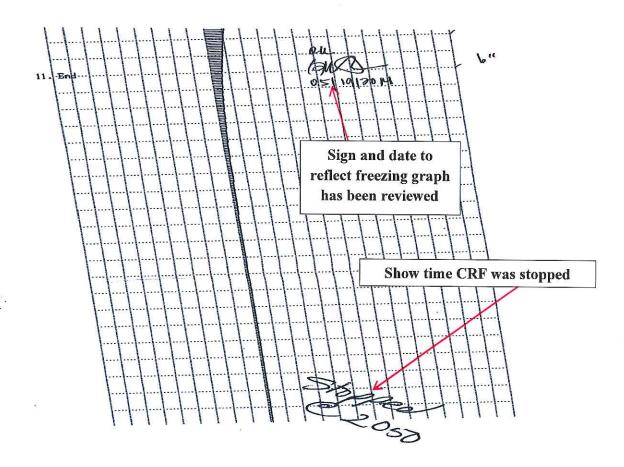
END - Holds **chamber** at -90°C until the CRF is stopped. Chamber stays at -90°C until BACK is pressed. Do <u>NOT</u> press BACK until you are ready to remove cryopreserved products from the Control Rate Freezer for storage in designated LN2 freezer.
