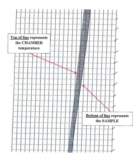
Step 8 – Continuation of step 8 (each horizontal line represents 1 minute (this screen shot spans a total of approximately 26 minutes).
